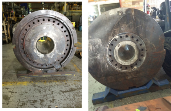
Heaters internal to container (left) and located close to liner (right)
