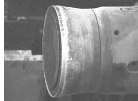
Figure 3-1: Fixed dummy block (Photo courtesy of Castool)
