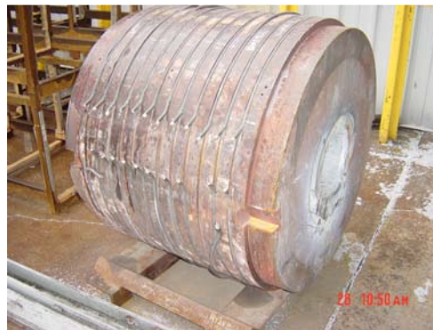
Figure 3-12: Container with external heating elements.
