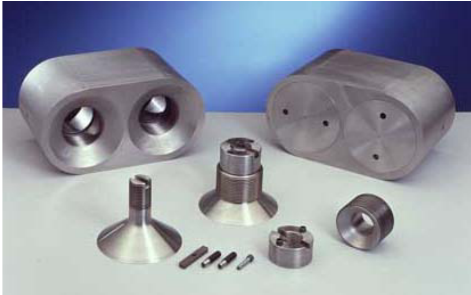
Figure 3-4: Fixed dummy block for oblong billet (Photo courtesy of COMPES)
