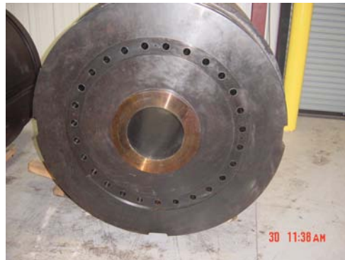
Figure 3-13: Container using heaters inserted into the mantle.
