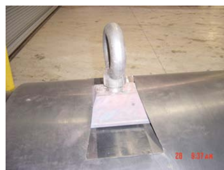
Figure 3-9: Alternative “dove tail” design for container lifting.
